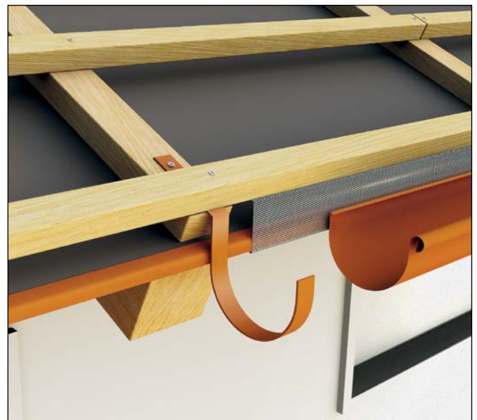
Option 1: Protection flashing going behind the gutter
