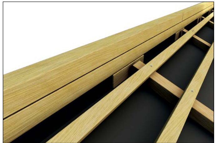
Option 2: Ridge batten - installation with batten understructure
