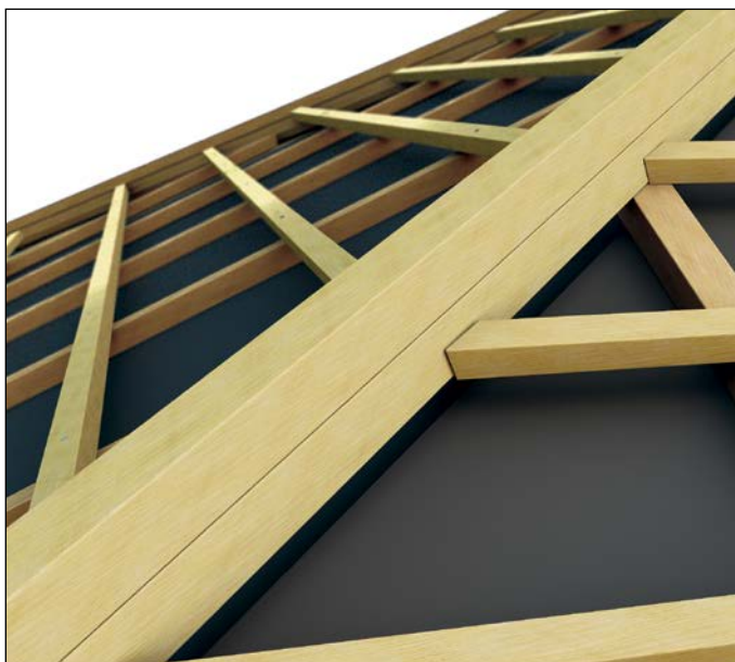
Option 2: Hip batten - installation with batten understructure
