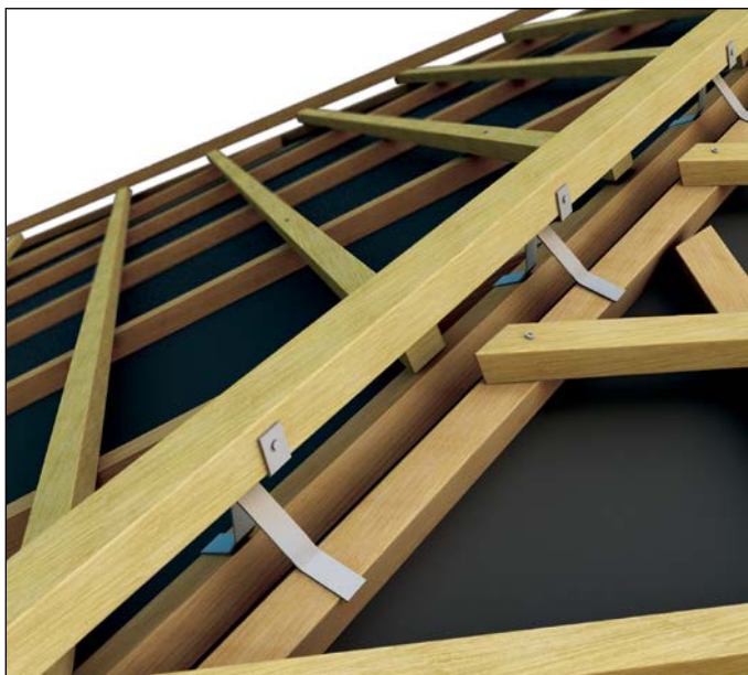
Option 1: Hip batten - installation with bracket
